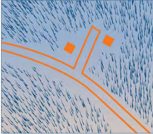
Inappropriate dead-end access
