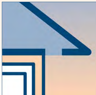
◀ Soffit vent too close to exterior wall
