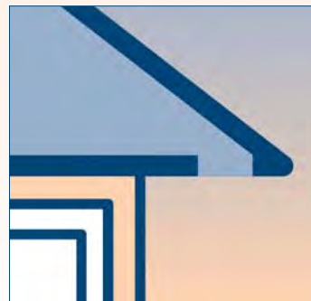
◀ Soffit vent too close to exterior wall
